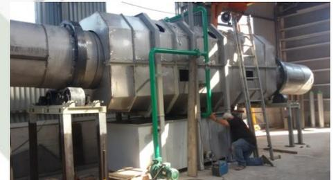
**Countercurrent rotary water coolers**, with some chambers inside the rotating drum for cold water and hot product. The water flows in its ducts in contact with the sides of the steel walls where the product is also in contact on the opposite side. This is necessary to transfer the energy from the warm side to the cold side.
