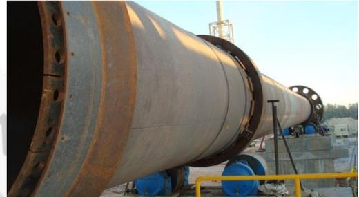
with a brick or castable lining, which protects the steel shell from the high internal temperatures. This kind of rotary kiln is a robust and efficient unit for heat transfer and pyroprocessing.
