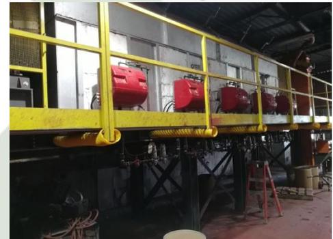
A benefit of the indirect rotary kiln is that because gas is not mixing directly with the material, much less gas is released from the shell, therefore requiring much less treatment of the expelled gases.
